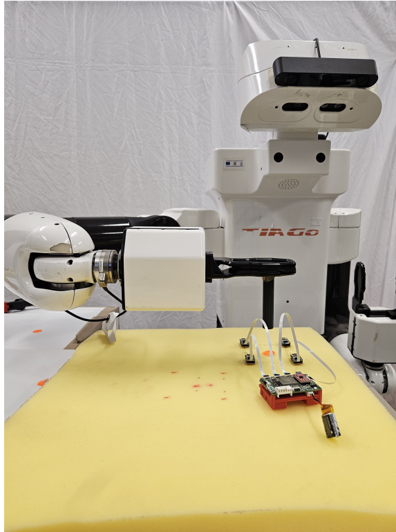
Figure 3.15: Complete set up before the actions start. TIAGo robot in position over the workspace, ready to impose the displacements. The sensors are positioned in the best-designed shape to detect such displacement.
