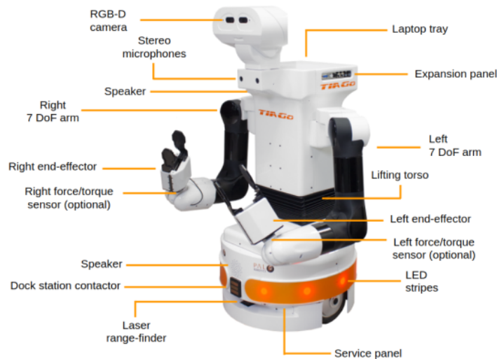
Figure 3.9: TIAGo robot and all its main components
