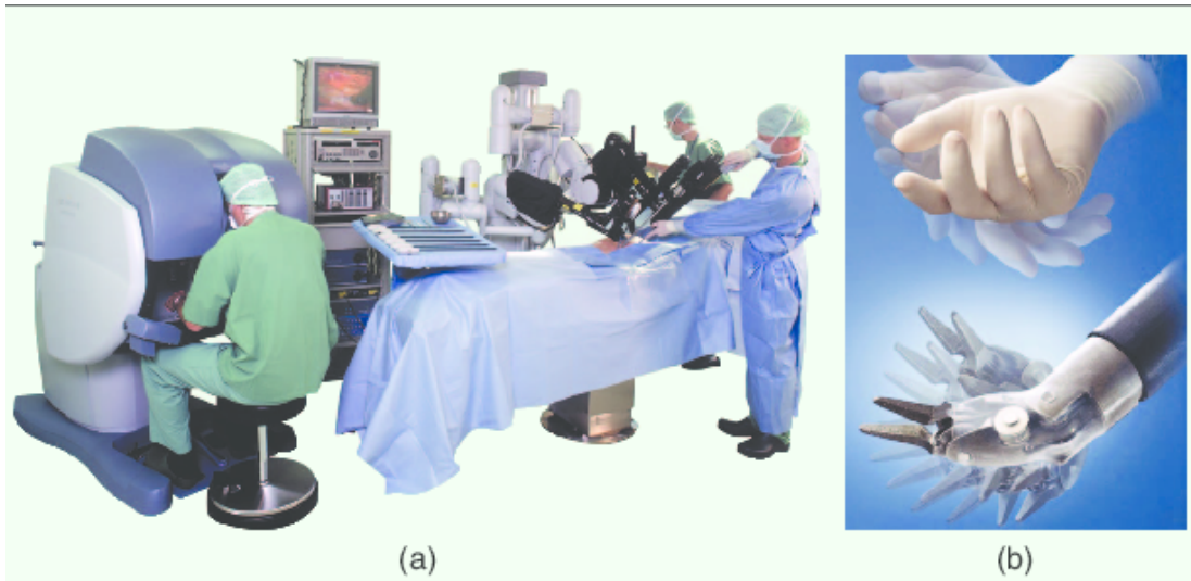
Figure 2.1: (a) The da Vinci surgical system consists of a master console and teleoperated patient-side robot. (b) Dexterous instruments enable fine manipulation inside the body. Okamura et al. (2010)
