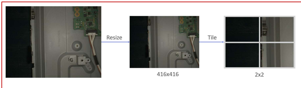
Figure 3.7: Original Image Being Resized and Tiled.
