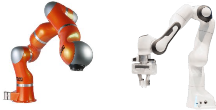
Figure 1.5 (left) Lightweight robotic arm Kuka LWR 4+, (right) Lightweight robotic arm Franka Emika Panda equipped with its standard gripper.
