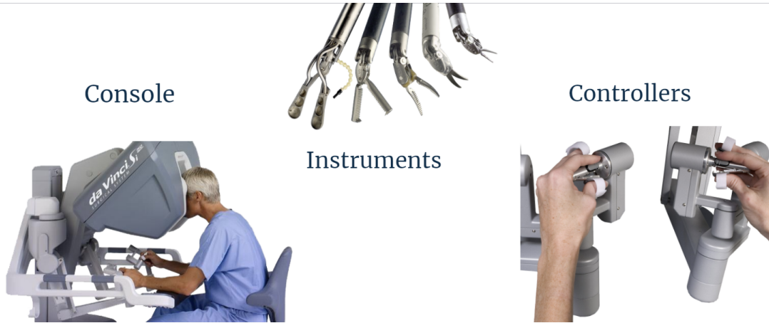
Figure 2.5: Console, controls and instruments of the daVinci robot
