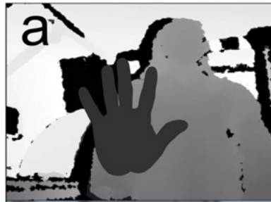
Figure 2.7: Depth image of a person performing a gesture with the hand (6)
