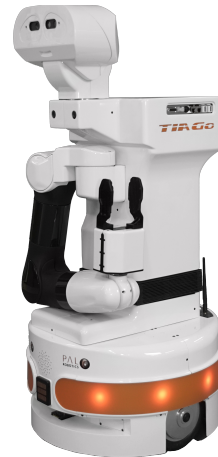
Fig. 1. The TIAGo service robot with its 7-DoF arm and a two-finger parallel jaw gripper manipulator. Both fingers will be equipped with tactile sensors for the newly proposed gripper configurations.
